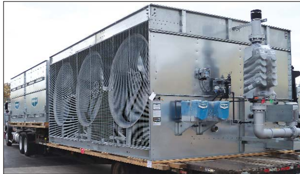
Evaporative Condenser Birmingham, AL USA
